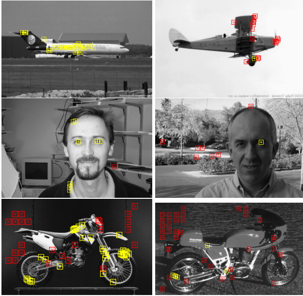
Figure 8: Typical examples of correct (left) and incorrect (right) classifications with positions of most discriminative patches for object (yellow) and background class (red).
