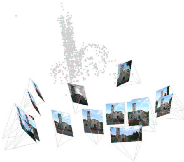
Fig. 11. VRML model of the scene computed for the Valbonne image set. Note that the distribution of images in the computed scene reflects the impression of proximity, adjacency etc that one gets by looking at the original images. There number of 3D scene points is 1034.
