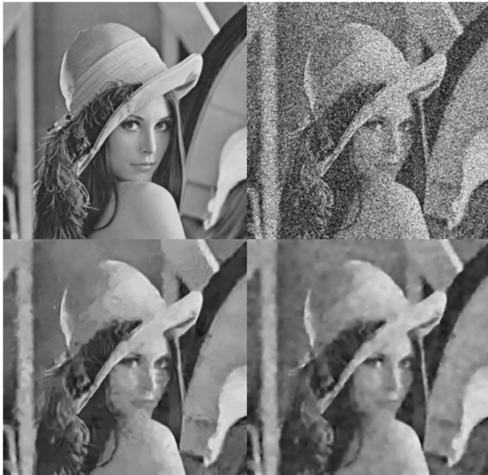
Fig.2. First row: “Lena” image and Lena with additive white Gaussian noise level \sigma = 100 ; Second row: results by BM3D and FLAD
