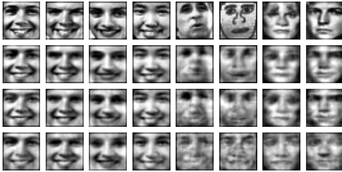
Fig. 8. Reconstructed images using the selected feature subsets. First row: original images; Second row: using top 50 eigenvectors; Third row: using the eigenvectors selected by SFBS; Fourth row: using the eigenvectors selected by GAs.
