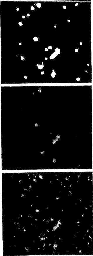
FIGURE 3.34 (a) Image of size 528 \times 485 pixels from the Hubble Space Telescope. (b) Image filtered with a 15 \times 15 averaging mask. (c) Result of thresholding (b). (Original image courtesy of NASA.)
