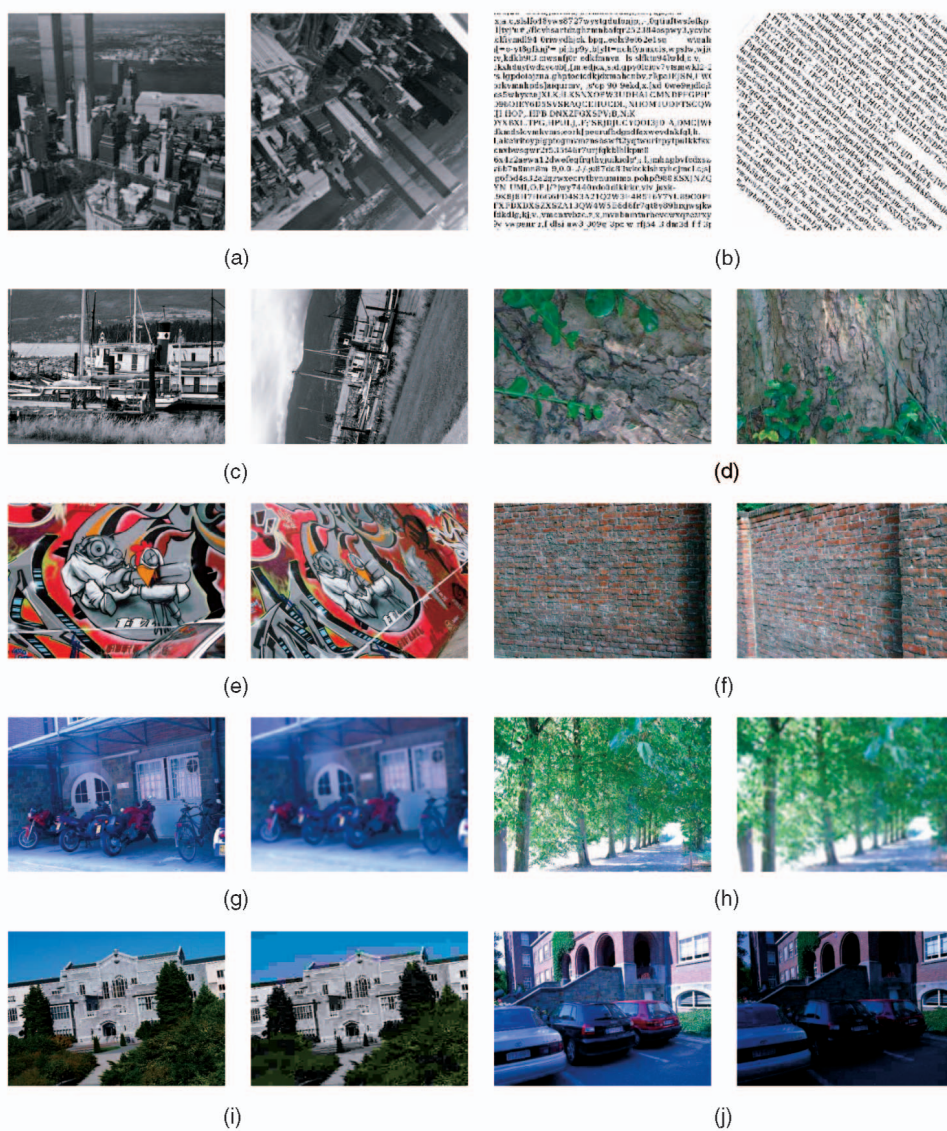
Fig. 3. Data set. Examples of images used for the evaluation: (a) and (b) rotation, (c) and (d) zoom+rotation, (e) and (f) viewpoint change, (g) and (h) image blur, (i) JPEG compression, and (j) light change.
