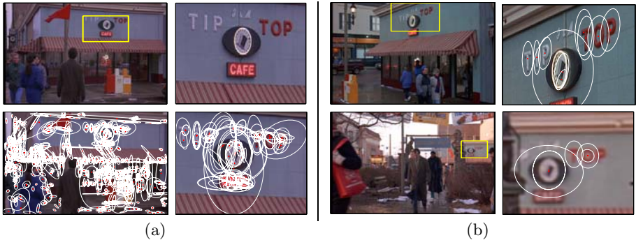
Fig. 1. Object query example I. (a) Top row: (left) a frame from the movie ‘Groundhog Day’ with an outlined query region and (right) a close-up of the query region delineating the object of interest. Bottom row: (left) all 1039 detected affine covariant regions superimposed and (right) close-up of the query region. (b) (left) two retrieved frames with detected regions of interest and (right) a close-up of the images with affine covariant regions superimposed. These regions match to a subset of the regions shown in (a). Note the significant change in foreshortening and scale between the query image of the object, and the object in the retrieved frames. For this query there are four correctly retrieved shots ranked 1, 2, 3 and 9. Querying all the 5,640 keyframes of the entire movie took 0.36 seconds on a 2GHz Pentium.
