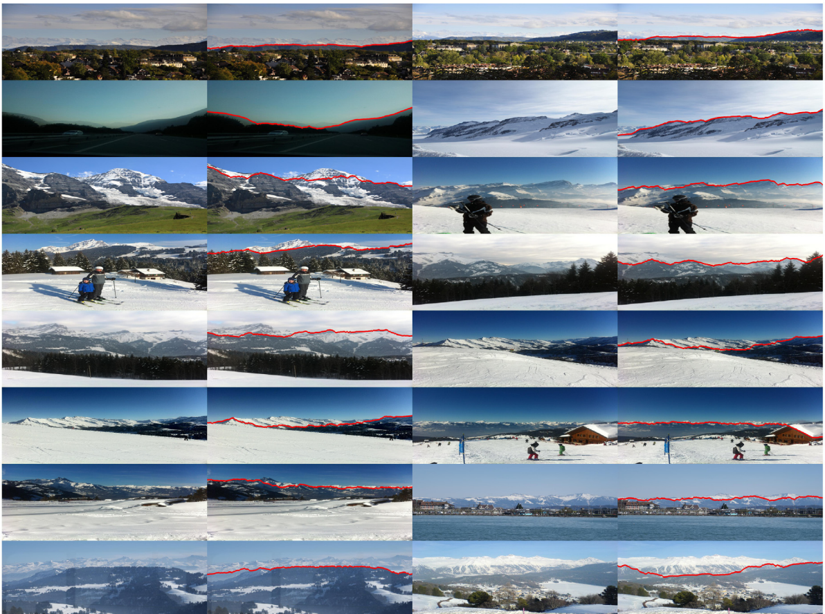
Fig. 15. Examples of faulty detection with average error more than five pixels: sample images (column 1 & 3), solution found by fusion approach (column 2 & 4).
