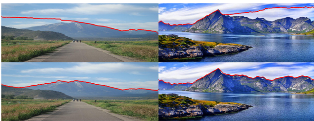
Fig. 7. Examples illustrating: [row 1] missing parts of the horizon line due to the assumption that the horizon line is close to the top of the image (Lie et al.), and [row 2] detecting the true horizon line using the proposed approach (SVM-mDCSI).
