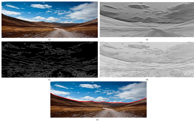
Fig. 13. Fusion based horizon detection: (a) query image, (b) DCSI, (c) MSEE Edges, (d) fused DCSI, (e) detected horizon (red boundary). (For interpretation of the references to color in this figure legend, the reader is referred to the web version of this article.)
