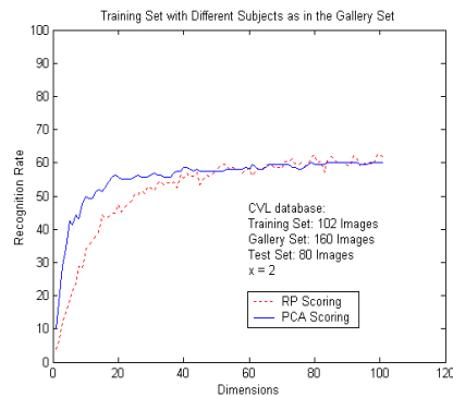
Figure 5. Experiments using the CVL database and scoring. The subjects in the training and gallery sets were different. The blue line corresponds to PCA using scoring, while the red line corresponds to RP using scoring. The proportion of subjects in the gallery and test sets varies as shown.
