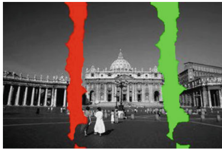
Fig. 10 Detection of original and duplicated regions using dense SIFT descriptors
