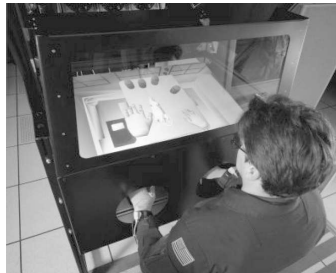
Fig. 1. Virtual Glove Box: A stereoscopic display station provides a high-resolution immersive environment corresponding to a glovebox facility. The users interact with virtual objects using datagloves.
