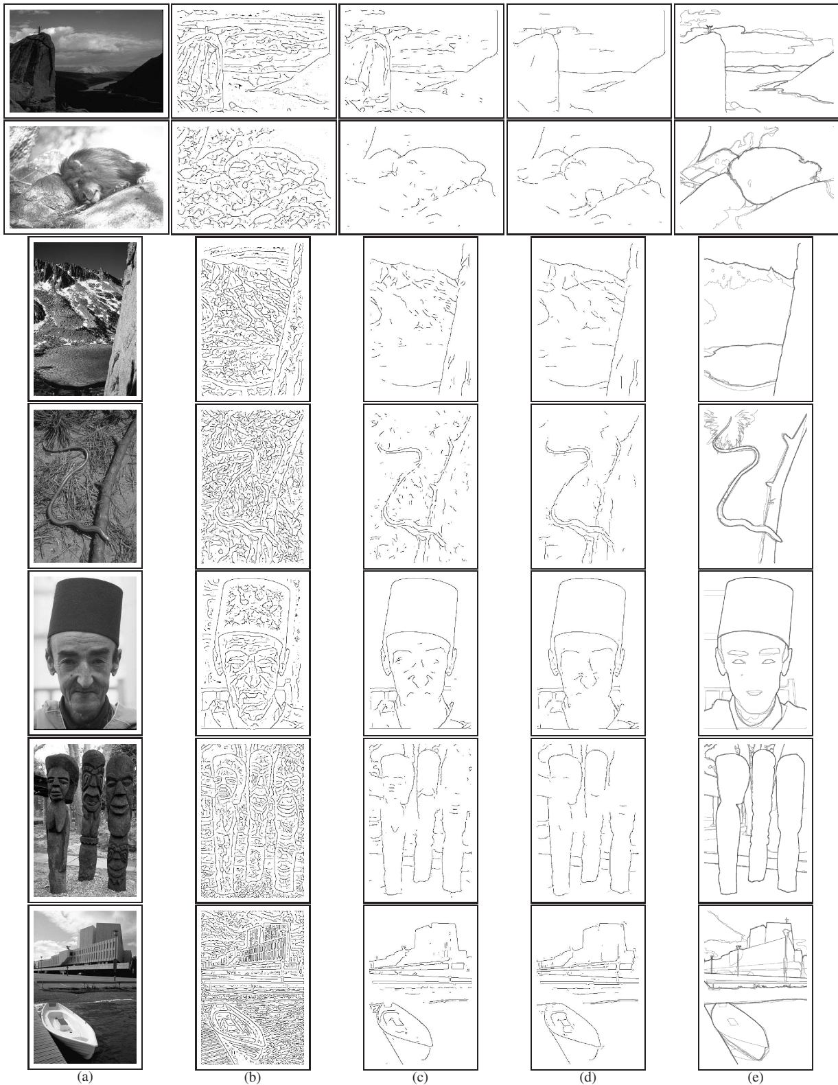
Figure 7. Visual comparison of results: (a) original grayscale images, (b) initial boundaries detected, (c) resulted boundaries by thresholding at the optimal F-measure (d) resulted boundaries using post-processing, thresholded at the optimal F-measure, (e) ground truth.
