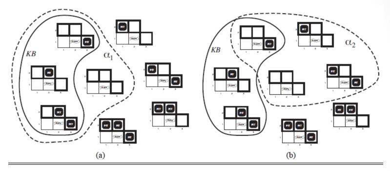
Figure 7.5 FILES: figures/wumpus-entailment.eps (Tue Nov 3 16:24:09 2009) figures/wumpusnonentailment.eps (Tue Nov 3 16:24:10 2009). Possible models for the presence of pits in squares [1,2], [2,2], and [3,1]. The KB corresponding to the observations of nothing in [1,1] and a breeze in [2,1] is shown by the solid line. (a) Dotted line shows models of  $\alpha_1$  (no pit in [1,2]). (b) Dotted line shows models of  $\alpha_2$  (no pit in [2,2]).
