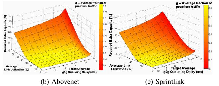
Fig. 3. MMPP/M/1 network model: The surface darkness shows the g2g target queuing delay. MMPP's burstiness is defined by  $a = 0.5$  and  $r = 4$ .
