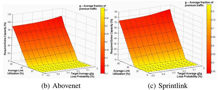
Fig. 4. MMPP/M/1/K network model: The surface darkness shows the g2g target loss probability. The buffer size is  $K = 60$  packets and the MMPP's burstiness is defined by  $a = 0.5$  and  $r = 4$ .
