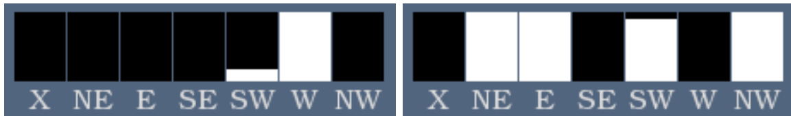
Figure 8.1: Output activations as confidence values. In these screenshots, a network’s output activations are shown graphically, with a vertical white bar showing each neuron’s activation value on a scale of [0, 1] and a symbolic code for the action-unit encoded interpretation beneath. Left: An output activation pattern plausibly interpretable as confidence values, with a high confidence for output option W , substantially less confidence for option SW , and no discernible level of confidence for any of the other options. Right: An output activation pattern only dubiously interpretable as confidence values, since over half the options are fully or near-fully activated. The network that produced these outputs was trained with deterministic winner-take-all decoding, and did not develop activation behaviors suitable for interpretation as confidence values.
