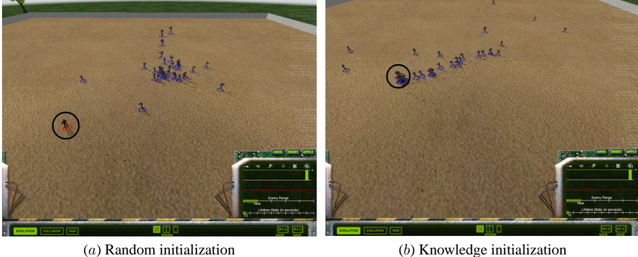
Figure 10: Testing Initial Behaviors to Approach a Single Roving Enemy. The environment contains a single roving enemy robot (circled). The rover circles the factory (cluster), from which the agents spawn. (a) With random neural network controllers, the agents run around in random fashion. (b) With controllers initialized with an FSM, they know how to approach the enemy right away. Alternatively, similar behavior can be discovered from the random behavior in (a) in about three minutes of rtNEAT evolution. Animations of these behaviors can be seen at http://nn.cs.utexas.edu/keyword?kbneat .
