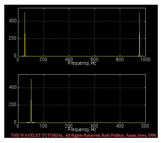
Figure 1.4 The FT of the 50 Hz signal given in Figure 1.3
