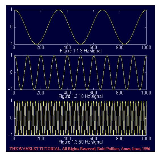
So how do we measure frequency, or how do we find the frequency content of a signal? The answer is **FOURIER TRANSFORM (FT)**. If the FT of a signal in time domain is taken, the frequency-amplitude representation of that signal is obtained. In other words, we now have a plot
