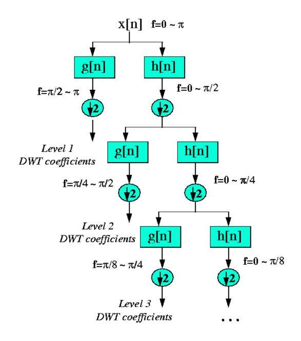
Figure 4.1. The Subband Coding Algorithm
