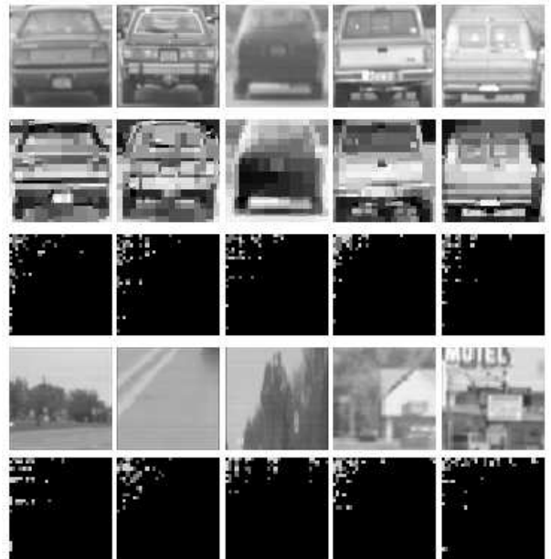
Fig. 5. 1st row: vehicle sub-images used for training; 2nd row: reconstructed sub-images using the 50 largest coefficients; 3rd row: illustration of the 50 quantized largest coefficients; 4th and 5th rows: similar results for some non-vehicle sub-images.
