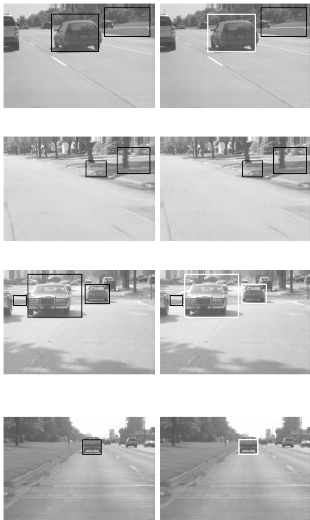
Fig. 4. Examples of the HG (left column) and HV (right column) steps: the black boxes indicate the hypothesized locations while the white boxes are the ones verified by the HV step.
