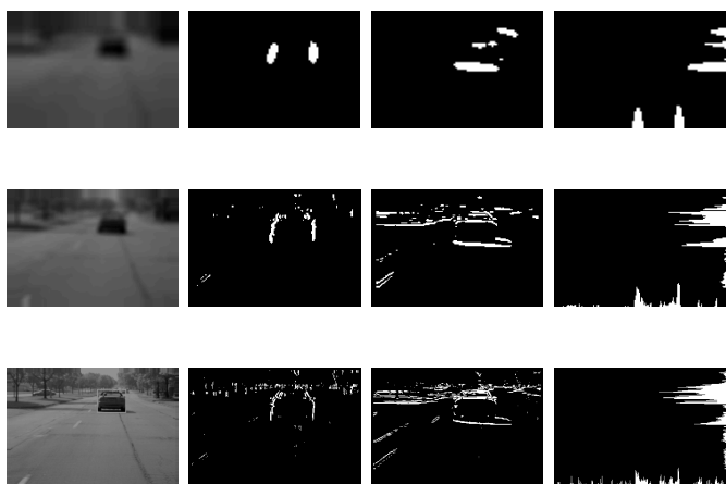
Fig. 3. Multi-scale hypothesis generation. The size of the images in the first row are: 90 \times 62 ; second row: 180 \times 124 ; and third row: 360 \times 248 . The images in the first column have been obtained by applying low pass filtering at different scales; second column: vertical edge maps; third column: horizontal edge maps; fourth column: vertical and horizontal profiles. Note that all images have been scaled back to 360 \times 248 for illustration purposes.
