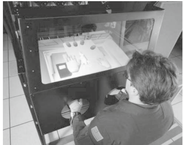
Fig. 1 VGX: A stereoscopic display station provides a high-resolution immersive environment corresponding to a glovebox facility
