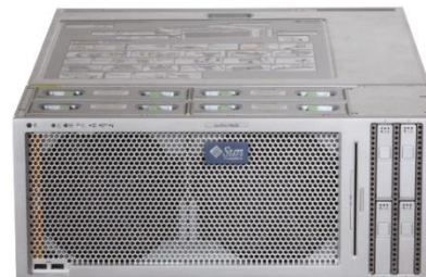
Sun 4600s and 4500s 16 core boxes with 200GB of RAM connected by Infiniband And several 24TB disk arrays
