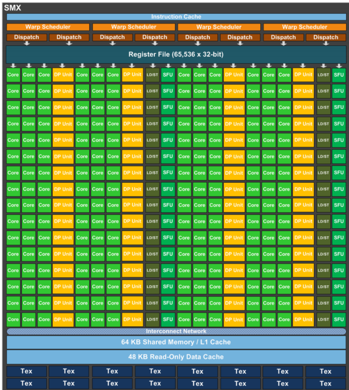
Figure 2.4: A block diagram of the Kepler architecture SMX[35]
