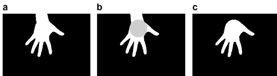
Fig. 9. (a) Binarized image, (b) largest circle that can be prescribed inside the hand–arm silhouette, and (c) segmented hand silhouette.
