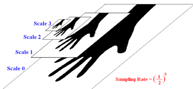
Fig. 8. Illustration of the multi-resolution hierarchy of hand images for reducing the computational cost of the hand–arm segmentation module. The hierarchy is obtained by down-sampling the binarized image three times, each time by a factor of two.
