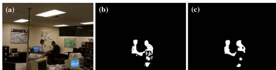
Fig. 9 Rapidly fluctuating background: a Handshake video sequence. b Detected foreground regions using AKDE. c Detected foreground regions using RM
