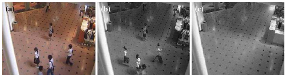
Fig. 12 Non-empty background: a Mall video sequence. b Background model after five frames using the RM method. c Background model after 95 frames using the RM method
