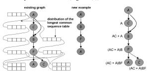
Figure 4: Incorporating new demonstrations: (a) Efficient computation of a generalized topology; (b) Behavior preconditions in a topological representation
