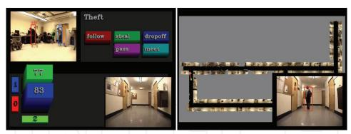
Fig. 2. An observer robot catches a human stealing a bag (left). The top left view shows the robot equipped with our system. The bottom right is the view of a patrol robot. The next frame (right) shows the patrol robot using vision and a map to track the thief.
