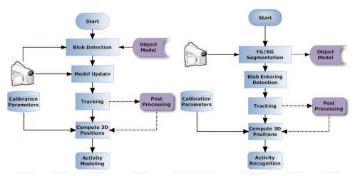
Fig. 1. The two object tracking frameworks for (a) *activity modelling* using a modified meanshift tracker and (b) *intent recognition* using a spatio-spectral tracker.
