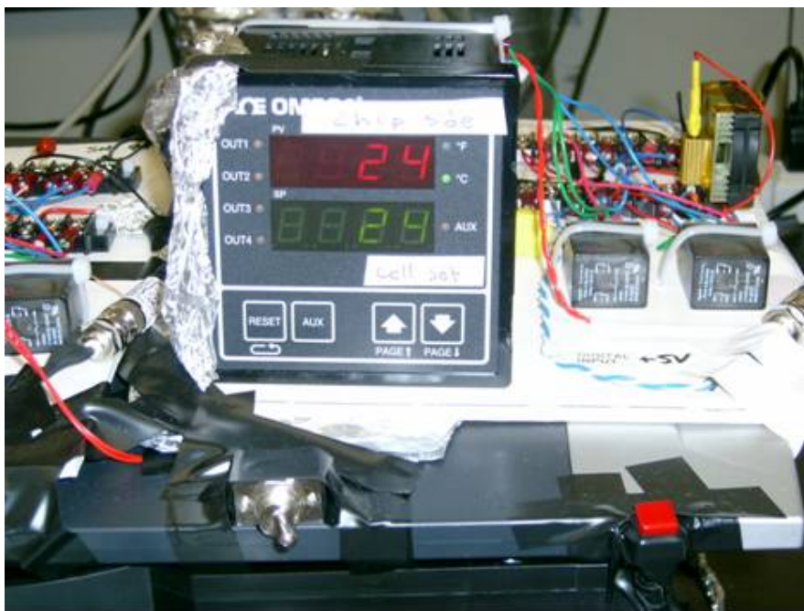
Figure 3. Temperature adjustment box for controlling the temperature of the array cell.
