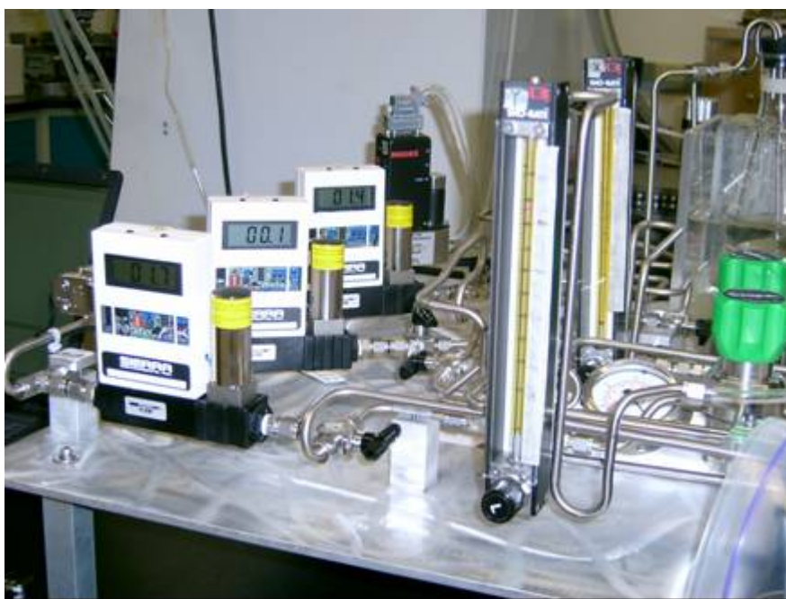
Figure 2. Flow rate control system for controlling the desired concentration of the chemical vapors.
