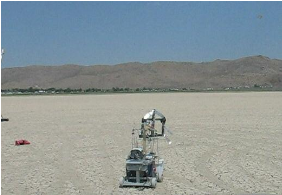
Figure 4-3 – Failed Complete Test Due to Blob-tracking Error
