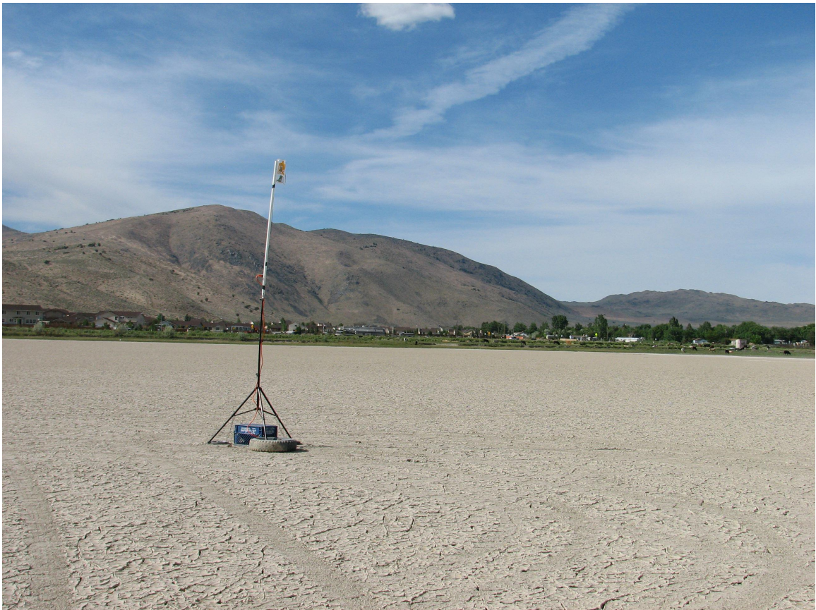
Figure 4-1 – Radio Tower Assembly Used to Mimic a Falling CanSat
