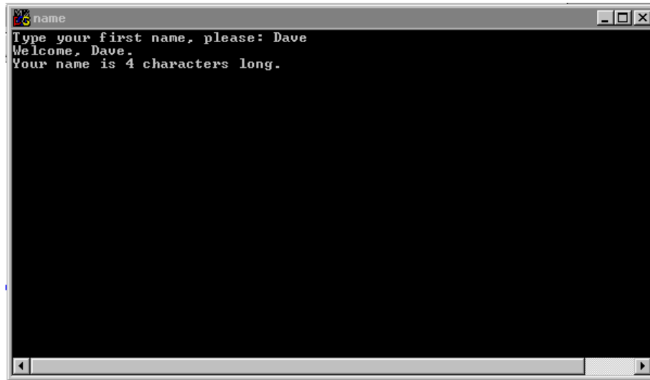
Figure 8.6 name prompts you to type in your name, then tells you how long your name is.
