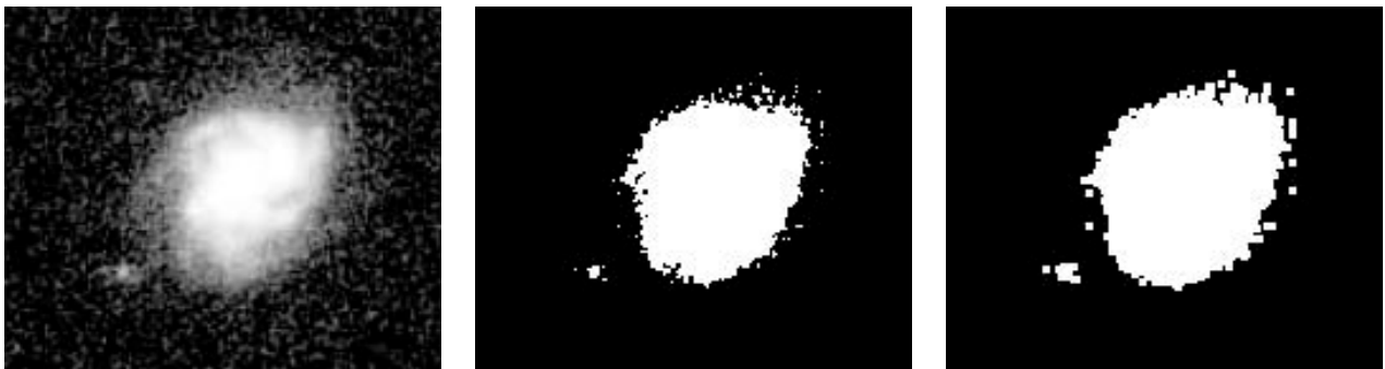
(a) (b) (c) Figure 3. (a) original image, (b) thresholded image, (c) dilated image.
