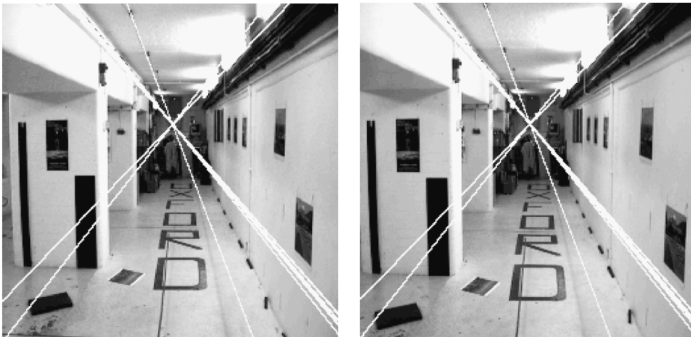
Fig. 4. Corridor scene. In the corridor scene the epipoles are right in the image.
