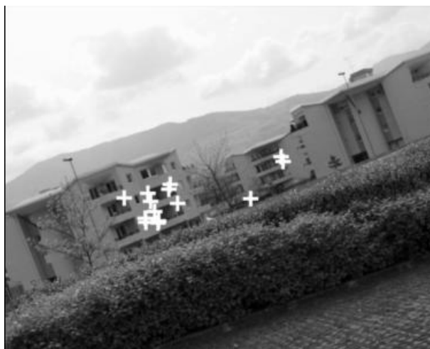
Figure 7: Example of images taken from different view points. There are 14 inliers to a robustly estimated fundamental matrix, all of them are correct. The estimated scale factor is 2.7.
