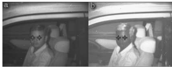
Figure 11: Example of our system detecting the driver of a car in an outdoor environment (a) Low near-IR image with the eye positions overlaid in green, (b) High near-IR image with the eye positions overlaid in green.
