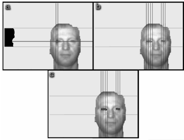
Figure 7: (a) The integral projection of a cross section in the lower band. The horizontal red line denotes the min location. (b) All of the lower band cross sections containing a substantive feature. (c) The grouping of adjacent substantive features into aggregate substantive features.
