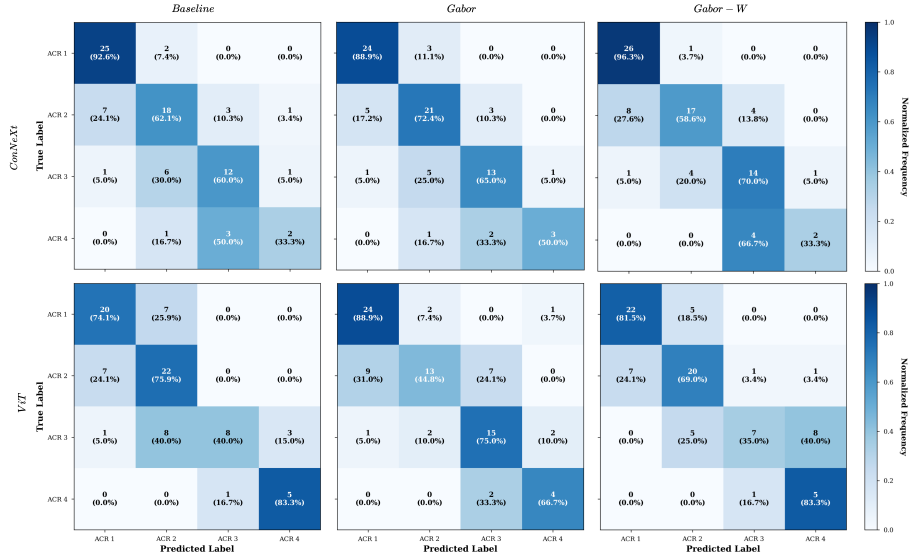
Fig. 2. Comparison of the confusion matrices of the proposed method with baseline using ViT and ConvNeXt. Confusion matrices for (left) baseline, (middle) proposed method (Gabor), and (right) pectoral muscle removed variant (Gabor-W).
