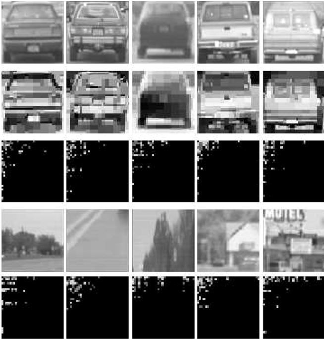
Fig. 8. First row: Vehicle subimages used for training. Second row: Reconstructed subimages using the 50 largest coefficients. Third row: Illustration of the 50 quantized largest coefficients. Fourth and Fifth rows: Similar results for some nonvehicle subimages.
