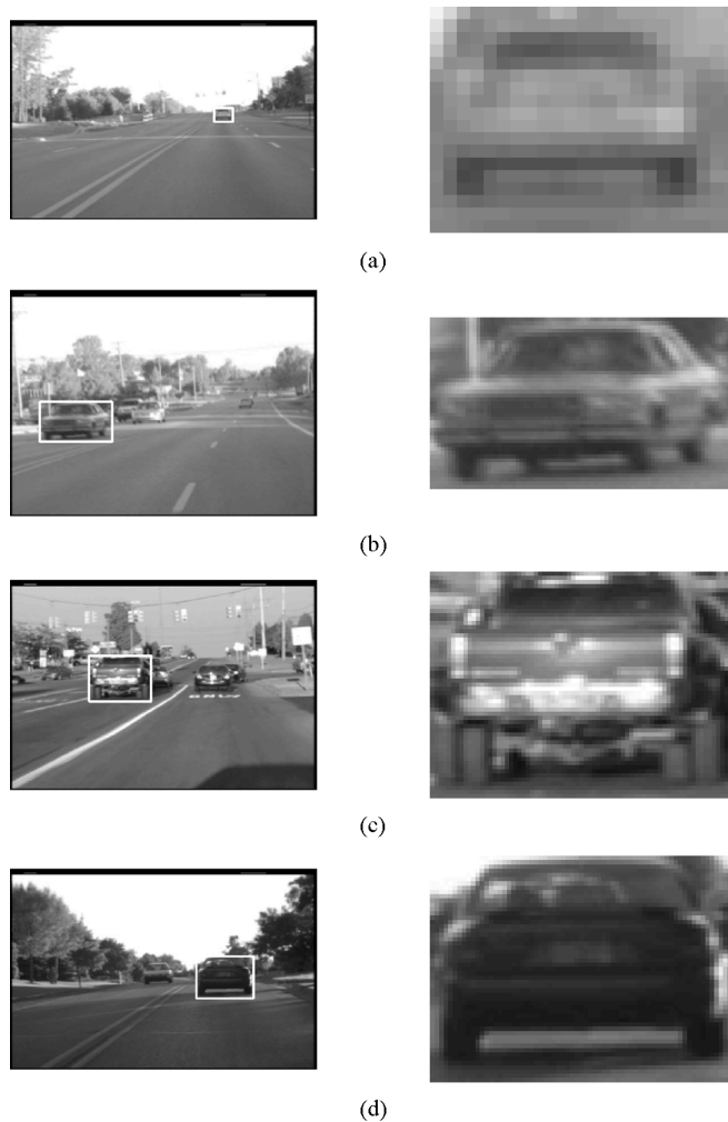
Fig. 14. Some examples of successful detection using Haar wavelet features (or Gabor features).
