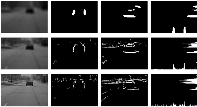
Fig. 5. Multiscale hypothesis generation. The size of the images in the first row are: 90 \times 62 ; second row: 180 \times 124 ; and third row: 360 \times 248 . The images in the first column have been obtained by applying low pass filtering at different scales; second column: vertical edge maps; third column: horizontal edge maps; and fourth column: vertical and horizontal profiles. Note that all images have been scaled back to 360 \times 248 for illustration purposes.
