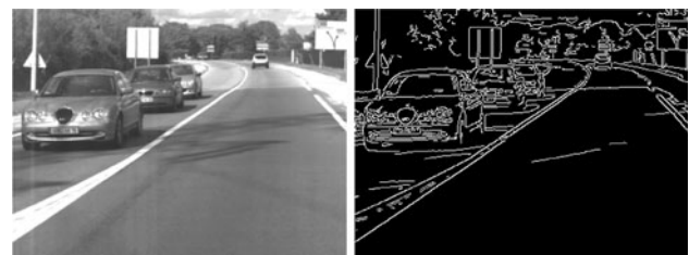
Fig. 12 ( left ) Left image #1983 of the real stereo sequence #2 and ( right ) the corresponding edge image obtained using the Canny edge detector
