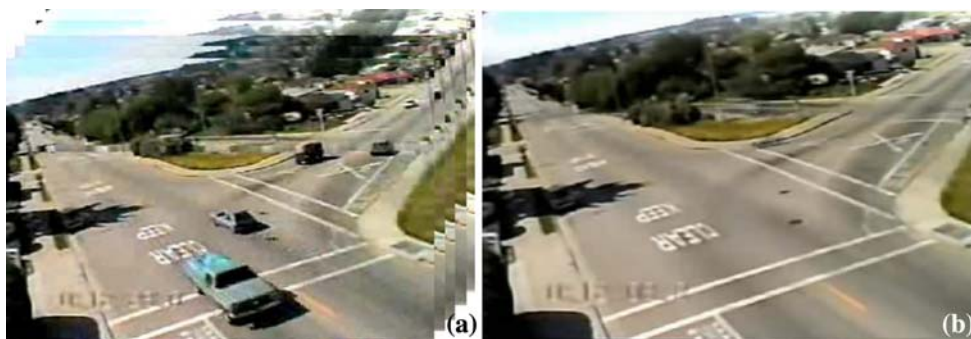
Fig. 2 Captured traffic scenes and the computed “clean” background scene using median filtering
