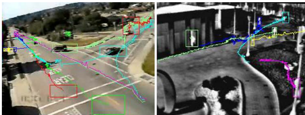
Fig. 15 Multiple target tracking and their trajectories. For each target, its trajectory is shown in the same color as its frame box
