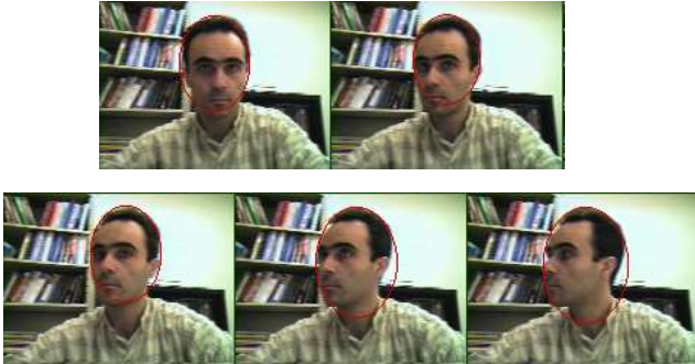
Figure 5. The elliptical head detector and tracker. The ellipses drawn around the head, show the detected locations of the head over a sequence of consecutive frames.
