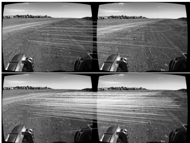
Figure 4. Visual feature matches between the current (right) and previous (left) frame using BRISK (top) and SURF (bottom) features.
