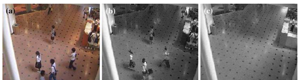
Fig. 12 Non-empty background: a Mall video sequence. b Background model after five frames using the RM method. c Background model after 95 frames using the RM method
