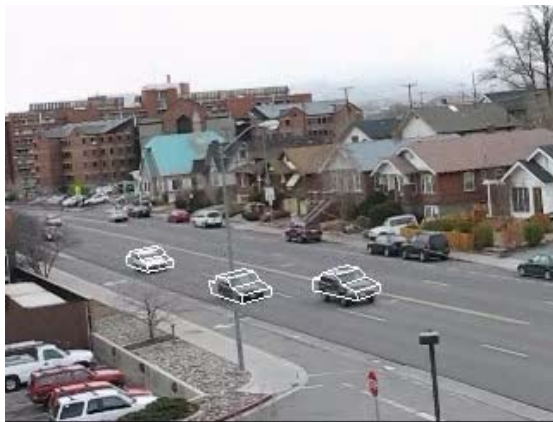
Fig. 5. Models overlapped onto actual vehicles (S1).
