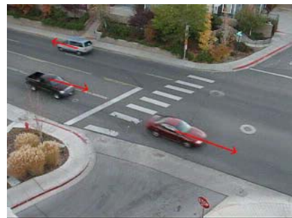
Fig. 2. Average optical flow vectors (red arrows).
