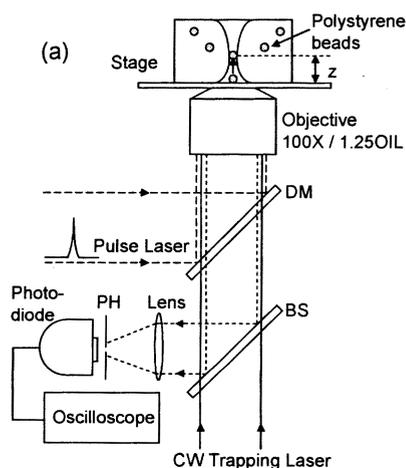
Fig. 1. Experimental Setup of pulsed optical tweezers
