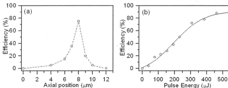
Fig. 4. (a) Levitation efficiency versus the initial distance ( $z$ ) in  $\mu\text{m}$  between the particle position laser focus (with a constant pulse energy of  $385 \mu\text{J}$ ). (b) Single pulse levitation efficiency versus pulse energy in  $\mu\text{J}$  at  $z=8 \mu\text{m}$ .
