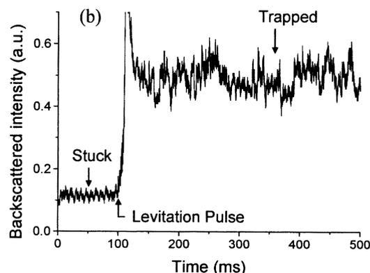
Fig. 2. Backscattered light intensity recorded at the detector as a stuck particle is levitated with an infrared pulse and jumps into the cw trap.
