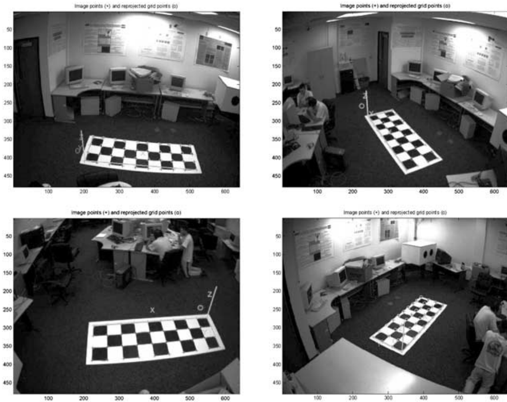
FIGURE 1. Illustration of setup for multiple camera calibration.
