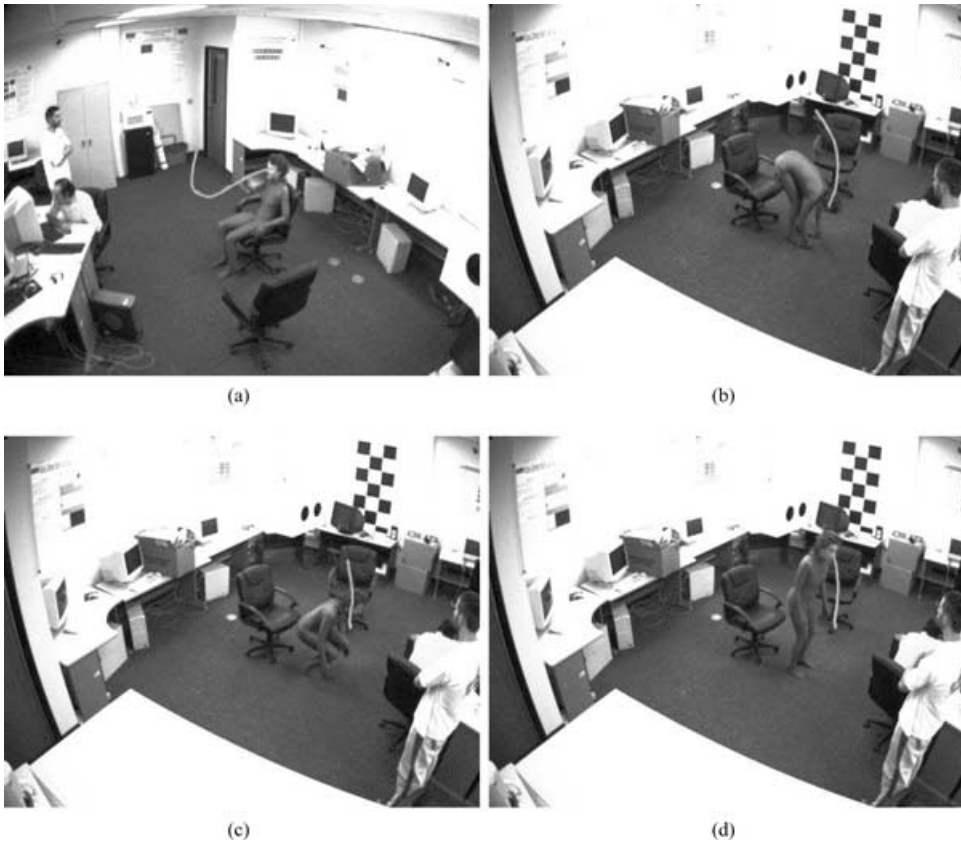
FIGURE 10. (a) Sitting-down at frame 123, (b) Bending-down at frame 177, (c) Squatting at frame 227, (d) Rising from squatting at frame 236. Once an action was recognized successfully, the 3D trajectory of that action was projected onto the last frame of the action for illustration purposes.
