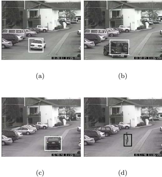
Fig. 7. Vehicle/pedestrian detection using the developed surveillance system: single presence
