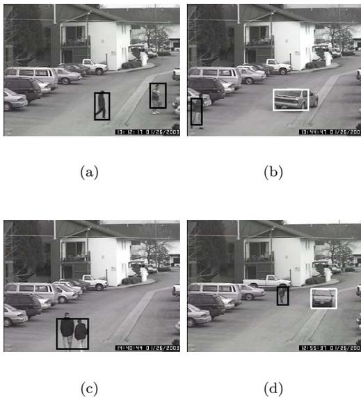
Fig. 8. Vehicle/pedestrian detection using the developed surveillance system: multiple presences
