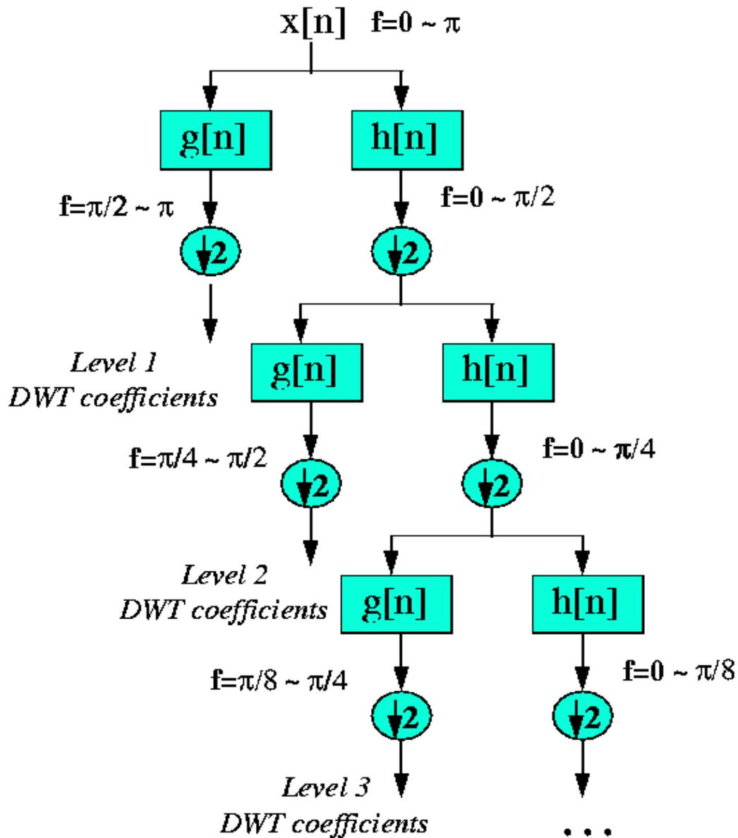
Figure 4.1. The Subband Coding Algorithm
