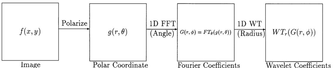
Fig. 1. Block diagram of the PFW algorithm.
