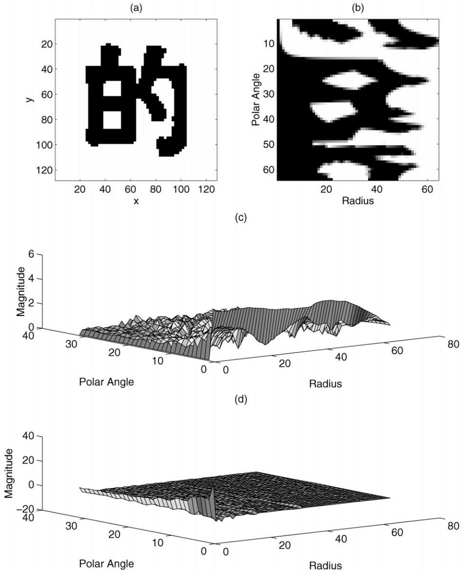
Fig. 2. An illustration of how a printed Chinese character is transformed after each step of the PFW algorithm. (a) The original printed Chinese character in Cartesian coordinates. (b) The polarized character in polar coordinates where each unit in the axis of the polar angle represents 6°. (c) The Fourier spectrum of the polarized character. (d) The wavelet coefficients based on the Fourier spectrum.
