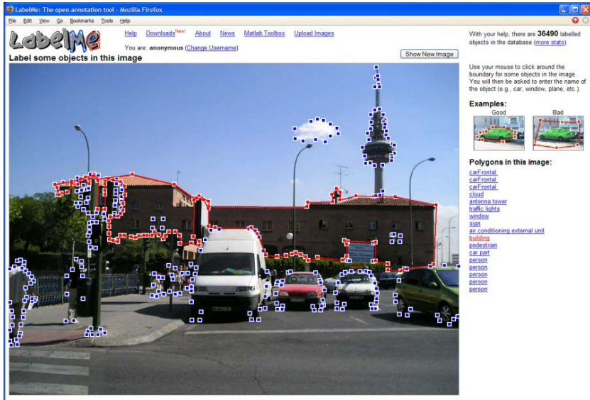
Fig. 9. Screenshot from the LabelMe labeling tool in use [25]. The user is presented with an image, possibly with one or more existing annotations in the image. The user has the option of annotating a new object, by clicking around the boundary of the object, or editing an existing annotation. The user can annotate an arbitrary number of objects in the image. Once finished, the user then clicks the “Show New Image” button to see a new image.
