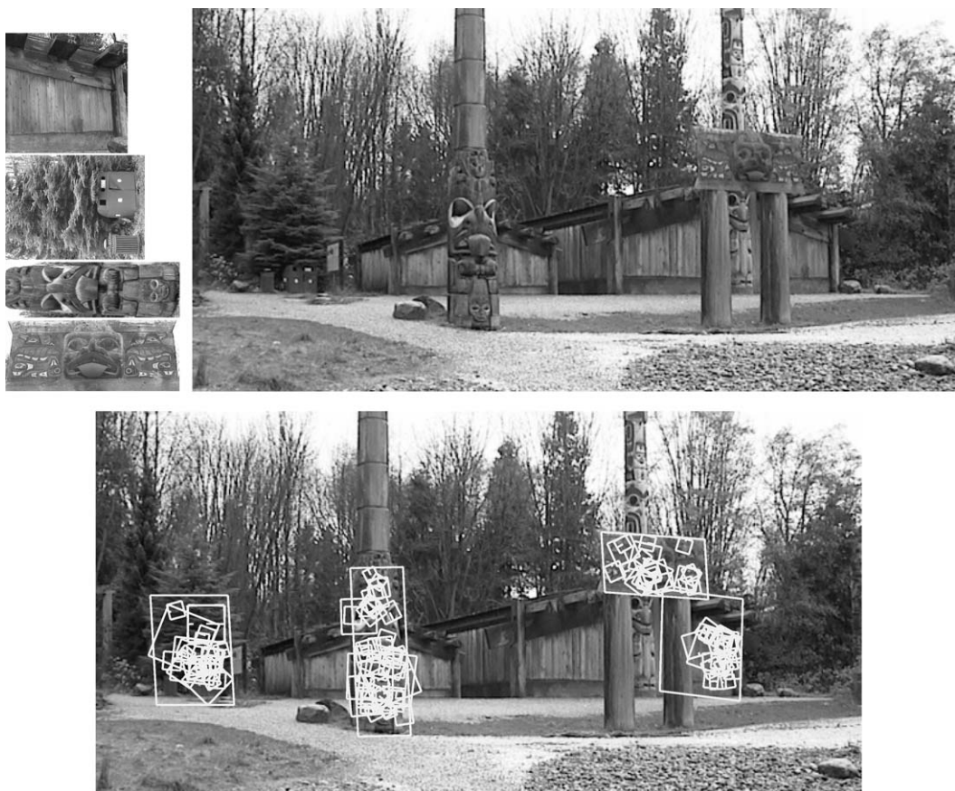
Figure 13. This example shows location recognition within a complex scene. The training images for locations are shown at the upper left and the 640 \times 315 pixel test image taken from a different viewpoint is on the upper right. The recognized regions are shown on the lower image, with keypoints shown as squares and an outer parallelogram showing the boundaries of the training images under the affine transform used for recognition.
