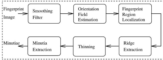
Fig. 7. Flowchart of the minutia extraction algorithm.
