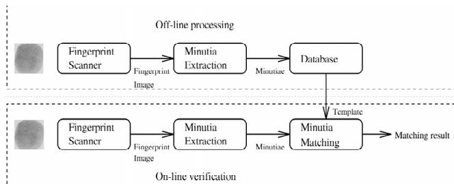
Fig. 6. Overview of our on-line fingerprint verification system.
