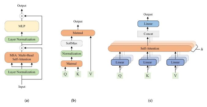
**Figure 2.** (a) The transformer block consists of an MSA, an MLP, skip connections, and layer normalizations. (b) Self-attention (Scaled Dot-Product Attention). Matmul: multiplication of two matrices. (c) Multi-head attention consists of multiple parallel self-attention heads. Concat: concatenation of feature representations. *h*: the number of self-attention heads.
