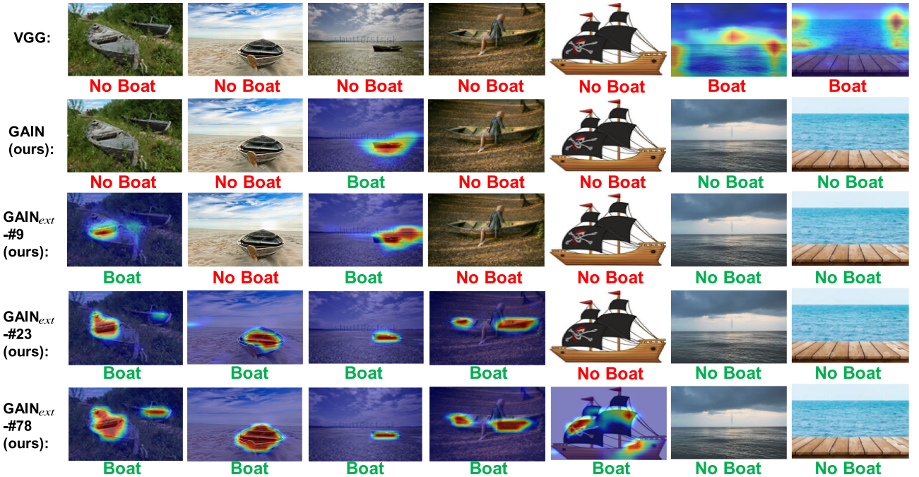
Fig. 7. Qualitative results generated by Grad-CAM [39], our GAIN and \text{GAIN}_{\text{ext}}^p on the Biased Boat dataset. -# denotes the number of pixel-level labels of boat used in the training which were randomly chosen from VOC 2012. Attention map corresponding to boat shown only when there are boats recognized.
